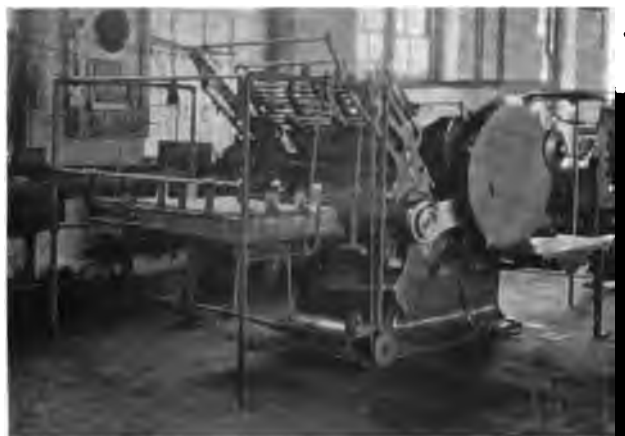
Fig. 4. Cutting and Creasing Press with Automatic Feed. (Pat.)
